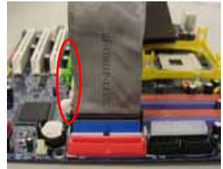
Fix the ODD cable to motherboard 將光碟機排線接至主機板
