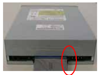
Fix the ODD cable to ODD 將光碟機排線接至光碟機
