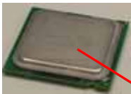
Evenly spread the heat dispersion paste on the CPU / 將散熱膏均勻塗抹於 CPU 上
