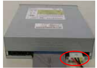
Fix the ODD cable to ODD 將光碟機排線接至光碟機
