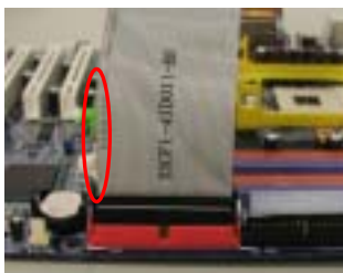
Fix the HDD cable to motherboard 將硬碟機排線接至主機板
