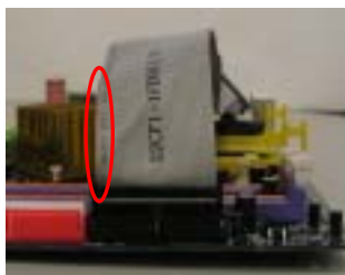
Fix the FDD cable to motherboard 將軟碟機排線接至主機板
