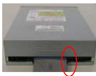
Fix the ODD cable to ODD 將光碟機排線接至光碟機
